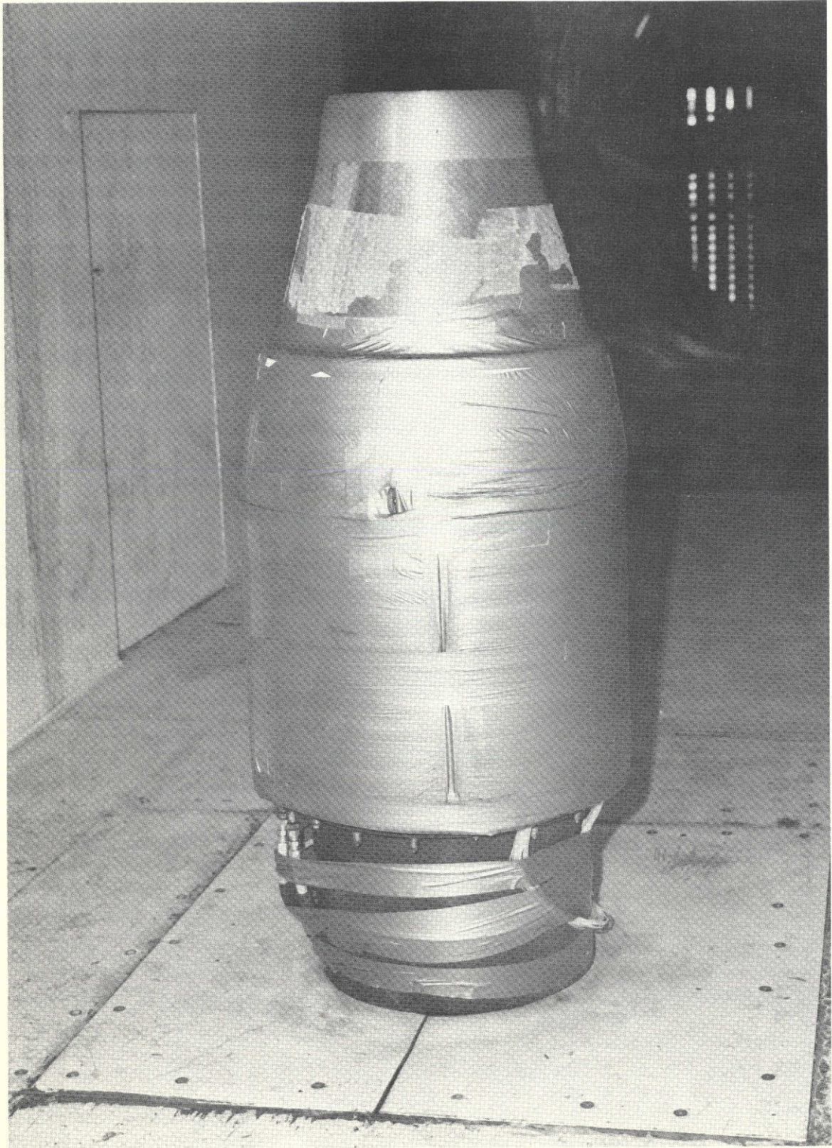
Figure 29.—Translating Centerbody Inlet A1 Takeoff— \alpha = 90^\circ
