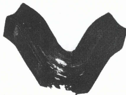
96 JOULES (71 FT-LB) 50 V/O 0.2 MM B IN 1100 Al (UNIDIRECTIONAL)
