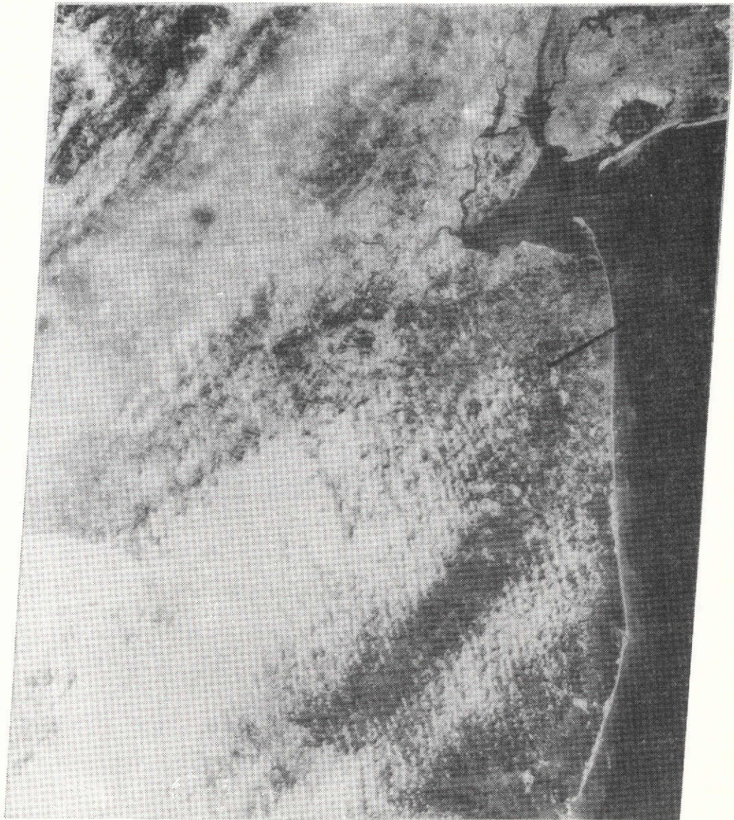
FIGURE 20. DREDGE SPOIL DUMPINGS, WHICH RANK FIRST IN BOTH TONNAGE AND COST OF ALL OCEAN DUMPED MATERIALS WERE LESS OFTEN IMAGED BY ERTS-1 THAN THE ACID WASTE DUMPS. DREDGE SPOIL DUMP SITES WERE GENERALLY FOUND CLOSER TO THE NEW JERSEY SHORE AND WERE GENERALLY LESS REFLECTIVE. NASA ERTS 1061-15125-5.
