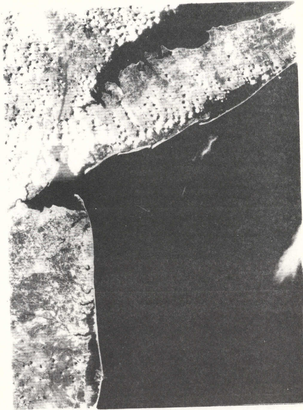
FIGURE 18. THIS MSS BAND 5 IMAGE TAKEN 16 AUGUST 1972 (1024-15071-5) CLEARLY ILLUSTRATES THE METHOD OF DUMPING THE HIGHLY REFLECTIVE ACID-IRON WASTE. THE BARGE DISCHARGES THE WASTE WHILE UNDERWAY AND WHEN HALF THE LOAD HAS BEEN DISCHARGED IT TURNS AROUND, DUMPING THE REMAINING LOAD. THIS PROCEDURE RESULTS IN THE CHARACTERISTIC HAIR-PIN PATTERN SEEN IN THE CENTER OF THIS IMAGE.
