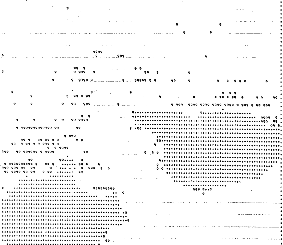
FIGURE 29 SAMPLE COMPUTER PRINTER OUTPUT 6-CYCLE RADIOMETRIC STRIPING PHENOMENON SANTA BARBARA CHANNEL 15 MARCH 1973 1/7 SCALE - DENSITY SLICE ON INTENSITY LEVEL 19 TO 19
