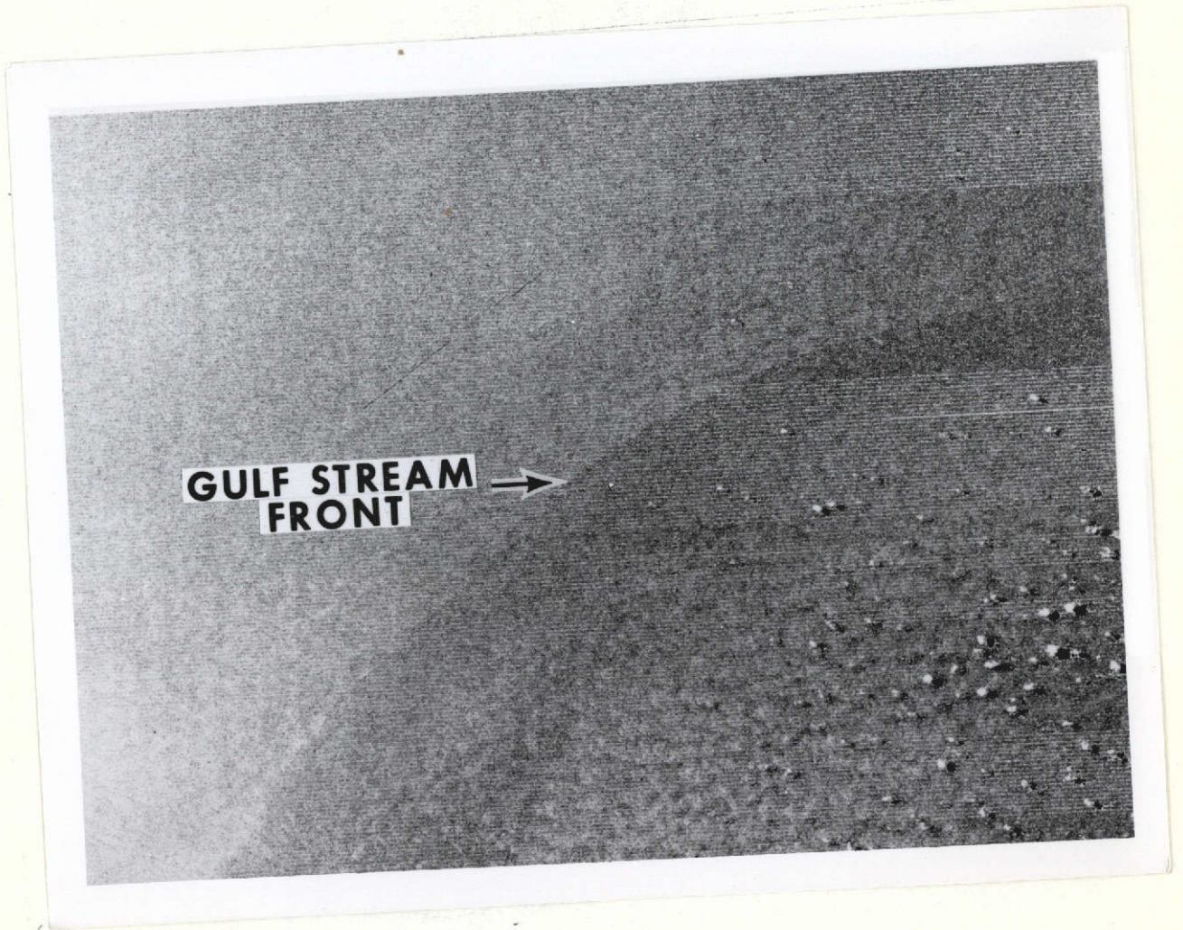
Figure A.17 Contrast stretched ( 11 \leq DN \leq 15 ; n=1 ) negative MSS 5 image of the Gulf Stream off Delaware (ERTS ID 1257-15033) observed on 6 April 1973. The stream is observable in this case due to higher radiance caused by increased sea state in the flow. This image is 350 km northeast of Cape Hatteras. There is a hazard in using sea state only to identify the current because even in MSS 7 a slight increase in radiance occurs which could be caused by high thin cirrus clouds. Horizontal distance across the image is 135 km.
