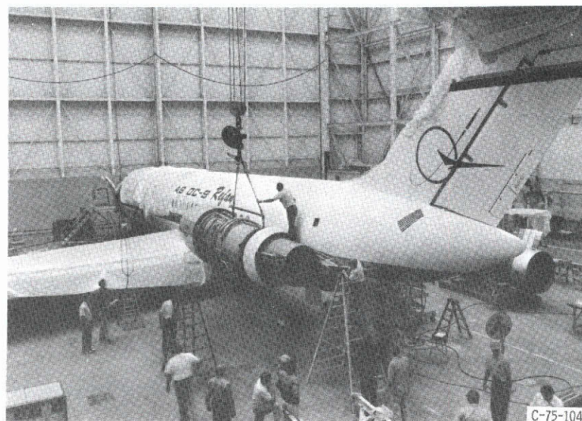
(d) Flight-test refan engine installation in DC-9 refan airplane at Douglas.
