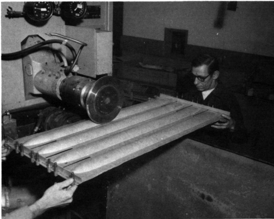
Figure 21: SEAM WELDING OF PANEL SUBASSEMBLY
