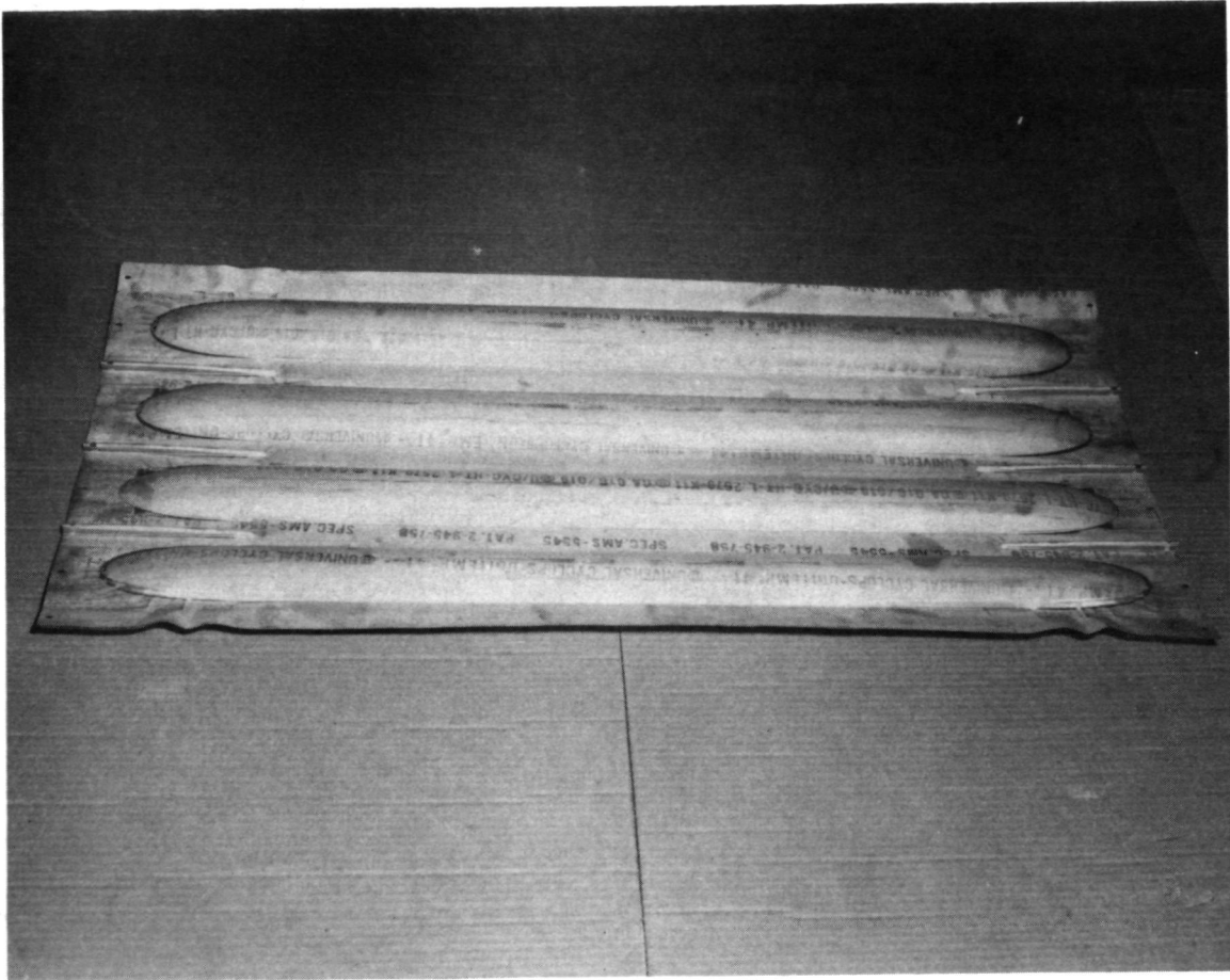
Figure 18: PANEL HALF WITH UNIFORM SECTION AND END CLOSURES FORMED
