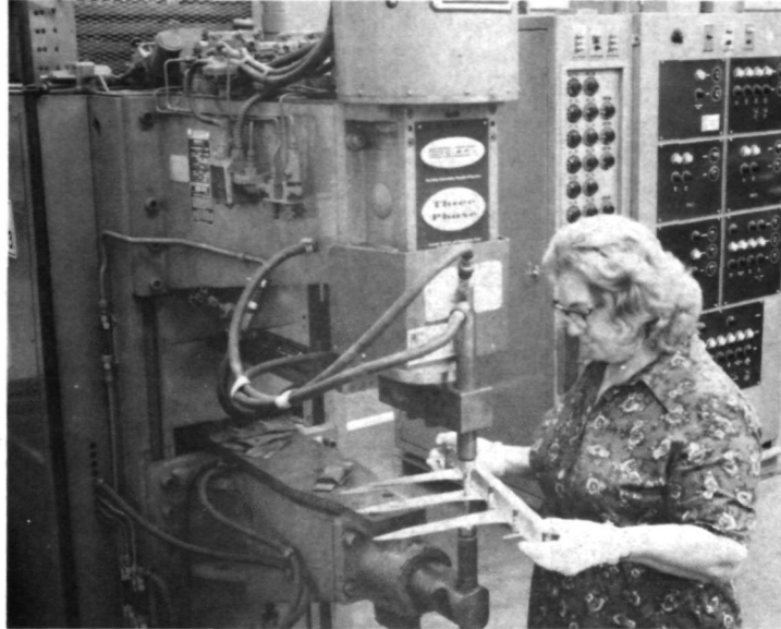
Figure 23: SPOT WELDING DOUBLER SUBASSEMBLY
