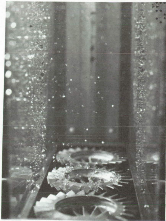
(b-2) Swirl-can design 2; fuel-air ratio, 0.02.
