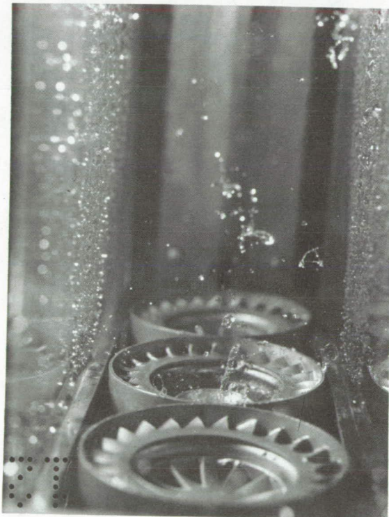
(b-4) Swirl-can design 6; fuel-air ratio, 0.026.
