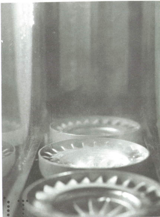
(a-3) Swirl-can design 5; fuel-air ratio, 0.026.
