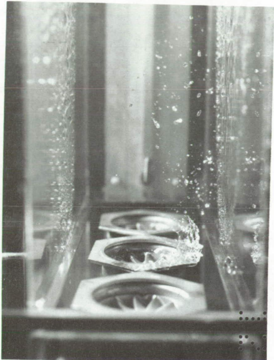
(b-1) Swirl-can design 1; fuel-air ratio, 0.02.
