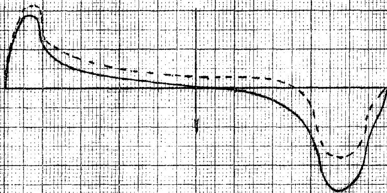
FIGURE 5.29c \Delta z for Antisymmetric Deflection. Rigid Wing Elastic Wing
