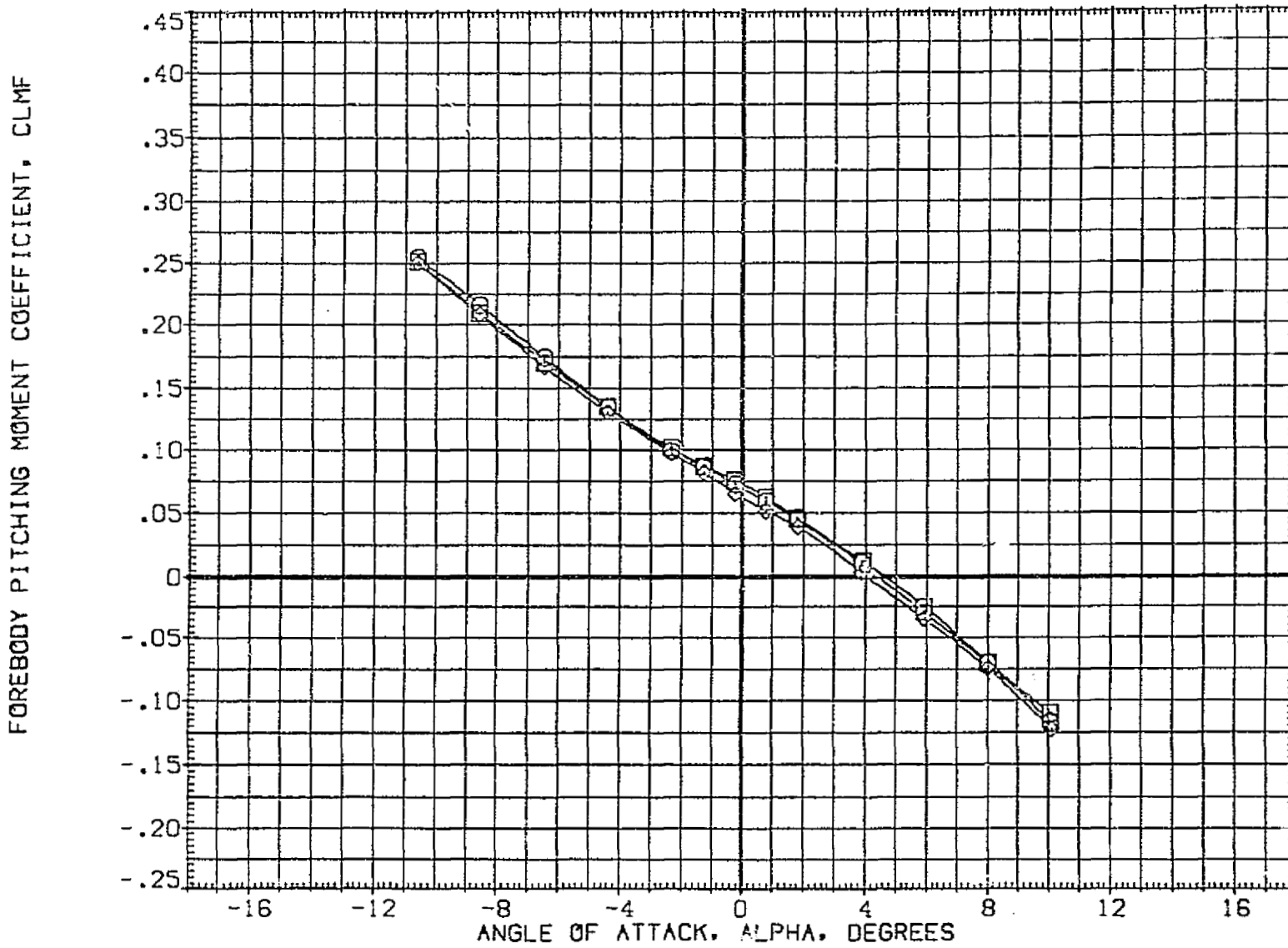
FIGURE 6 EFFECT OF BETA ON LAUNCH VEHICLE LONG. CHARACT. (C)MACH = 2.86
