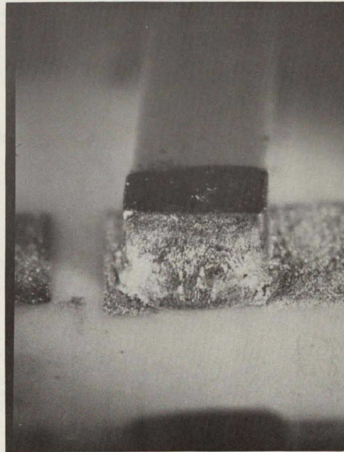
b. Bonding pad metallization peel from substrate. Typical when fillet bridges from capacitor to bonding pad edge.
