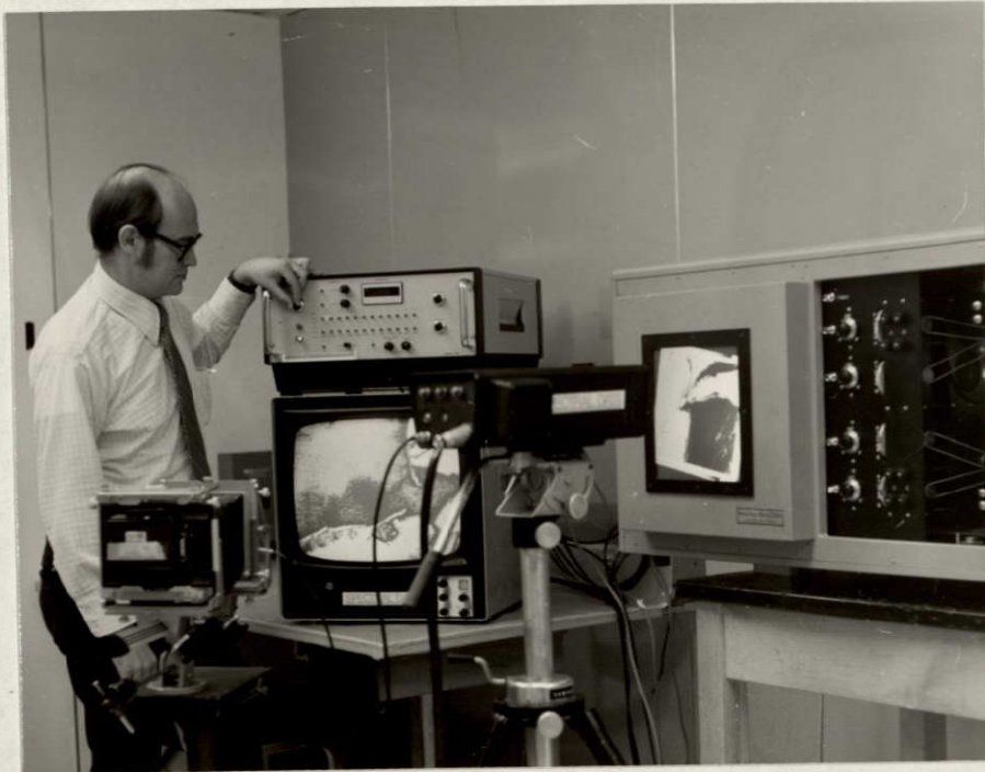
Figure 8. Spectral Data additive color viewer and Spatial Data density slicer used together to analyze ERTS imagery.
