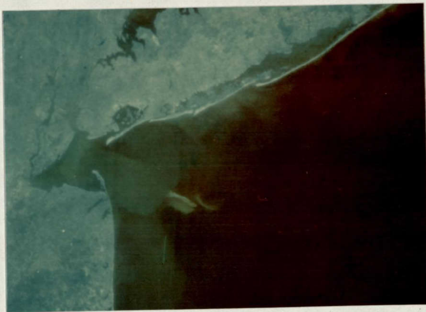
Figure 12. Multispectral rendition of ERTS MSS bands 4, 5, and 6 taken on 7 April 1973. Band 4 projected as red, band 5 as green, and band 6 as blue.
