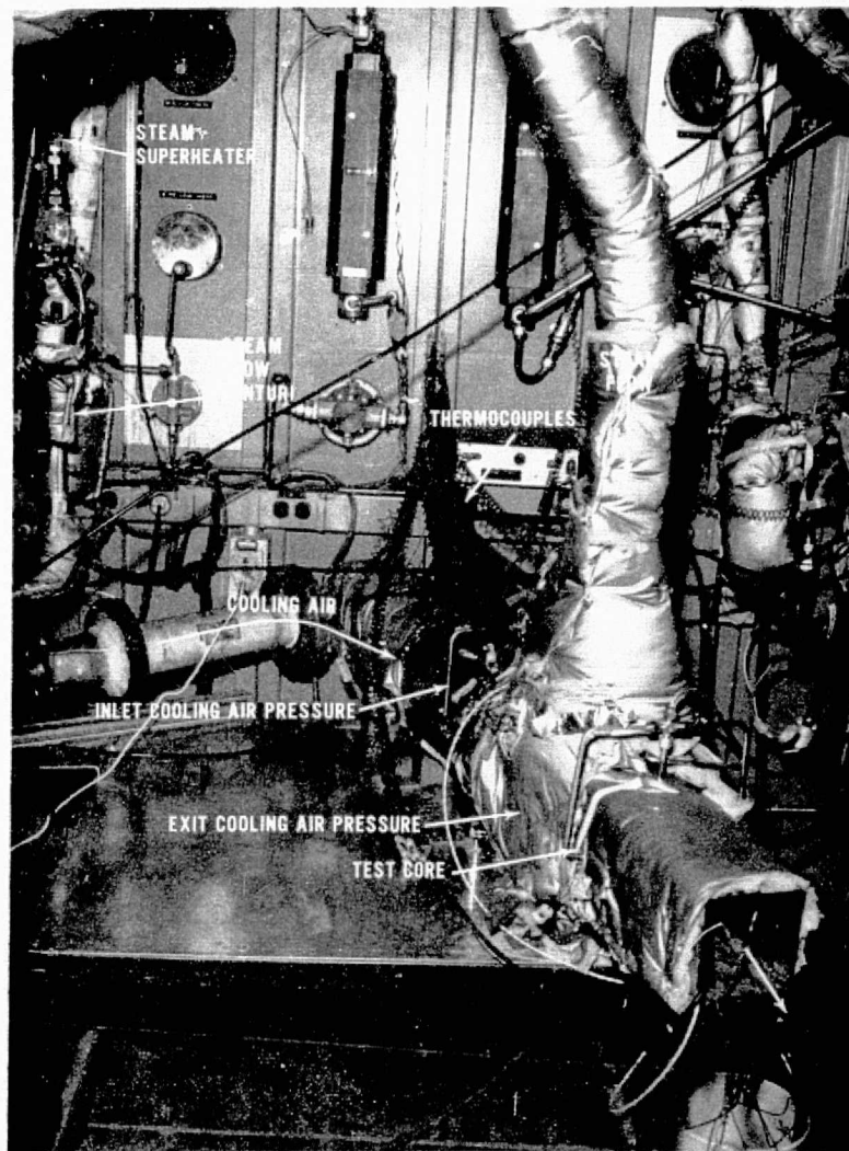
Figure 59 – Heat Exchanger Test Stand
