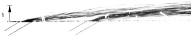
Figure 10. - In-line, 30^\circ injection into a thick boundary layer.
