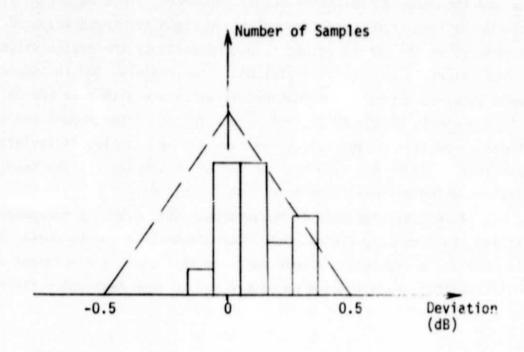
FIGURE A-1 SPACECRAFT ANTENNA GAIN: NUMBER OF SAMPLES VS. DEVIATION
