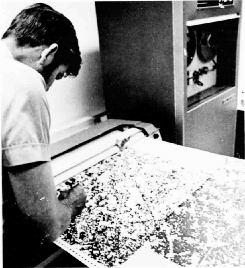
(a) Cal-Comp Plotter Drawing a Category on Mylar
