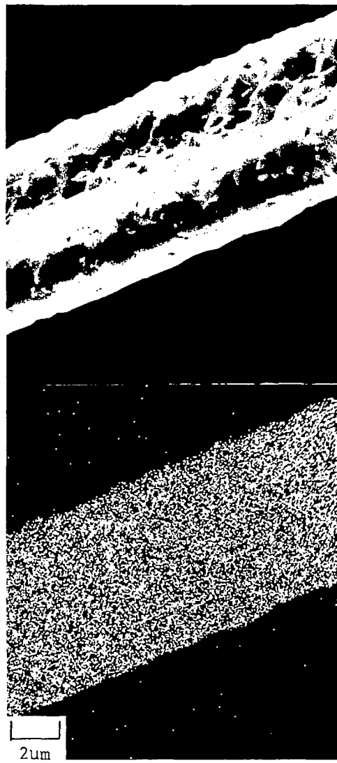
Fig. 1b. SEM specimen images (top row) and Ti x-ray images (bottom row) of Thornel 50 fibers CVD-coated with TiC for 60 min at 1473 K (run 5-6-74), 1723 K (run 5-10-74), and 1973 K (run 5-16-74). Coating gases contained no \text{CH}_4 .
