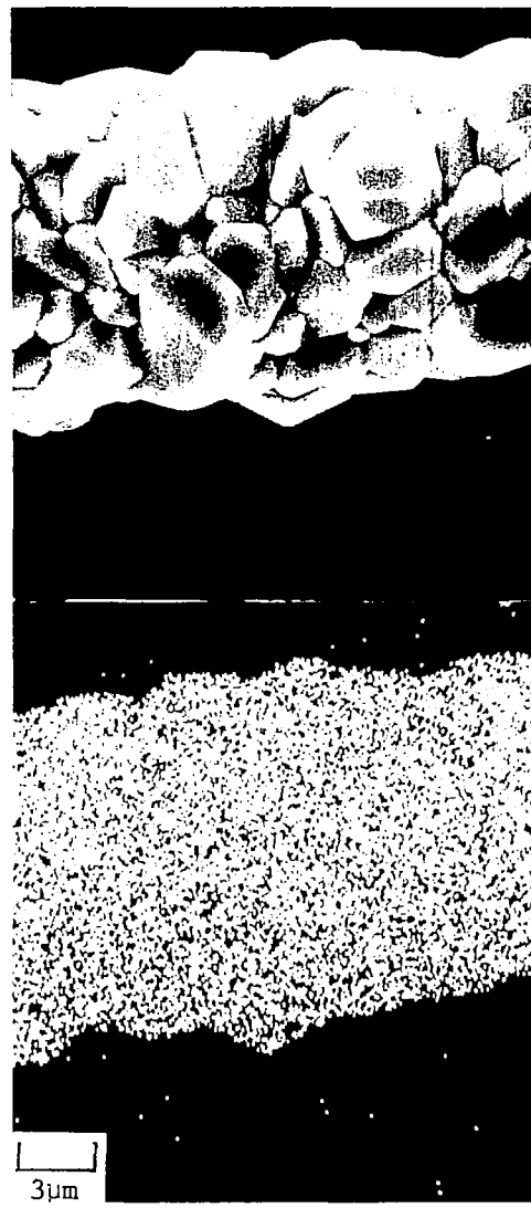
Fig. 1b. SEM specimen images (top row) and Ti x-ray images (bottom row) of Thornel 50 fibers CVD-coated with TiC for 60 min at 1473 K (run 5-6-74), 1723 K (run 5-10-74), and 1973 K (run 5-16-74). Coating gases contained no \text{CH}_4 .
