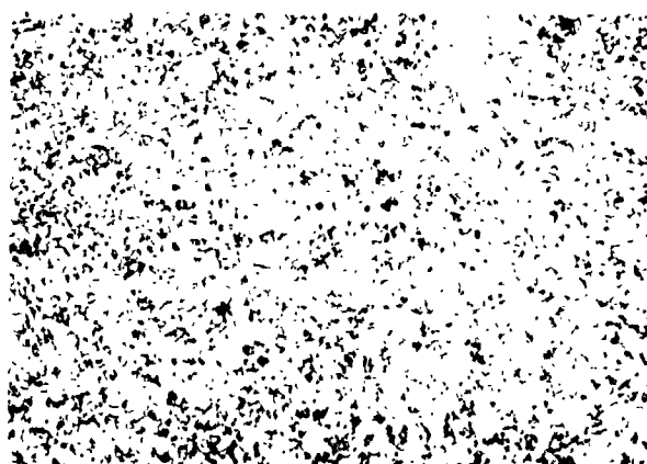
Figure 3. Typical microstructure of INCOLOY alloy 903 in the solution-treated and age-hardened condition. Etchant: Glyceregia 100X.
