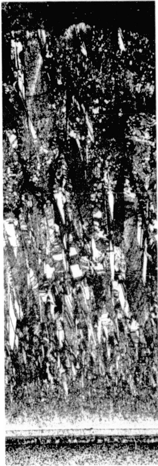
Figure 38. Microstructure of Sputtered OFHC Copper Deposited at 700°K (800°F) and 19.7 nm/s (2.8 mils/hr), Run II-7
