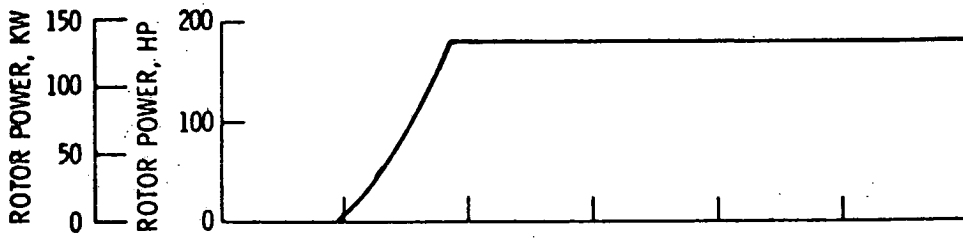
Figure 3. - ROTOR POWER AS A FUNCTION OF WIND SPEED
