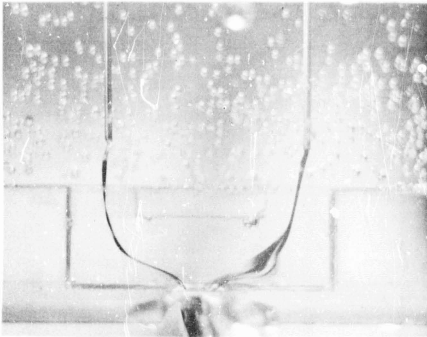
Figure 31.a Streak Lines (1.0 gal/min)
