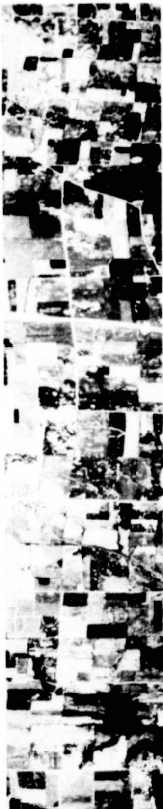
Figure 2. Aircraft Multi-spectral Scanner imagery (.58-.65 \mu band) showing severe geometric distortion due to crosswinds. LARS Run No. 71054100. Area is immediately west of Crawfordsville, Indiana. Date: August 17, 1971. Altitude: 5,000 ft.
