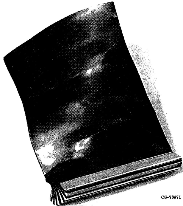
Figure VII-6. - PMR polyimide/graphite fiber fan blade.
