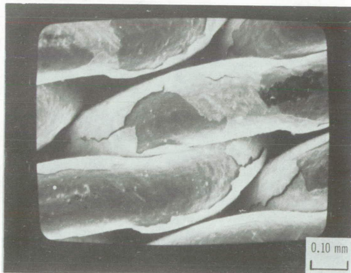
Figure 29. - Electron micrograph of stainless-steel screen anode insert (after test), showing spalled coating areas and cracks.
