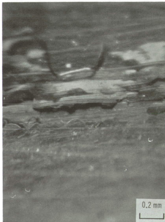
Figure 23. - Photomicrograph of deposits near upstream end of thruster body interior surface after test.
