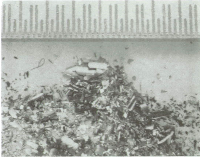
Figure 18. - Portion of loose flakes and material collected from thruster discharge chamber after test. Smallest divisions on ruler, each 0.254 millimeter (0.01 in.).
