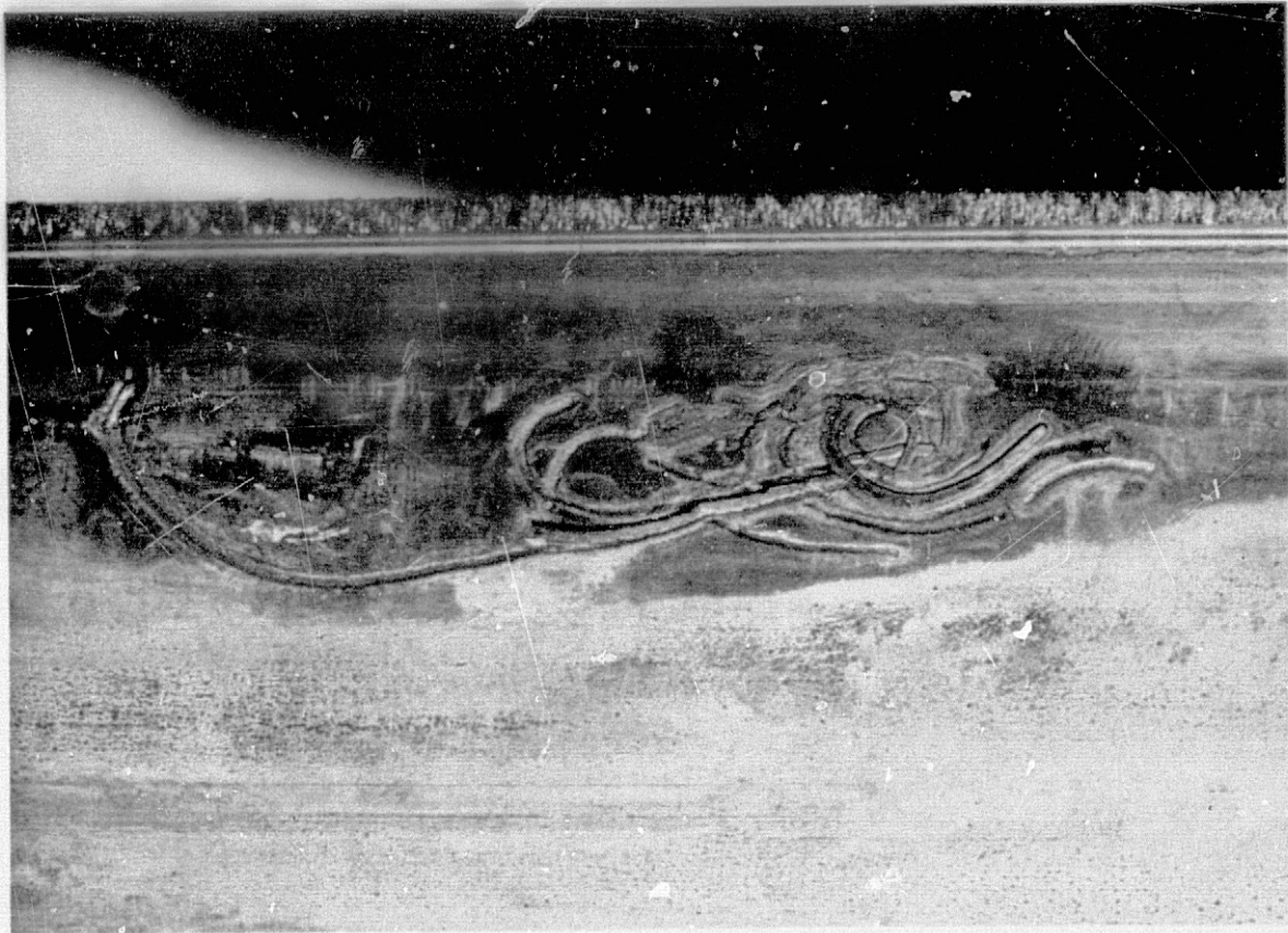
Figure 34. Closeup of imbedded chip
