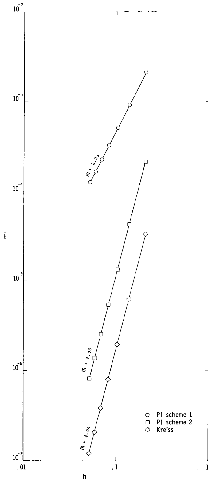
Figure 4.- Average errors from solutions to Burgers' equation for \nu = 1/8 . (The abbreviation PI indicates partial implicitization.)
