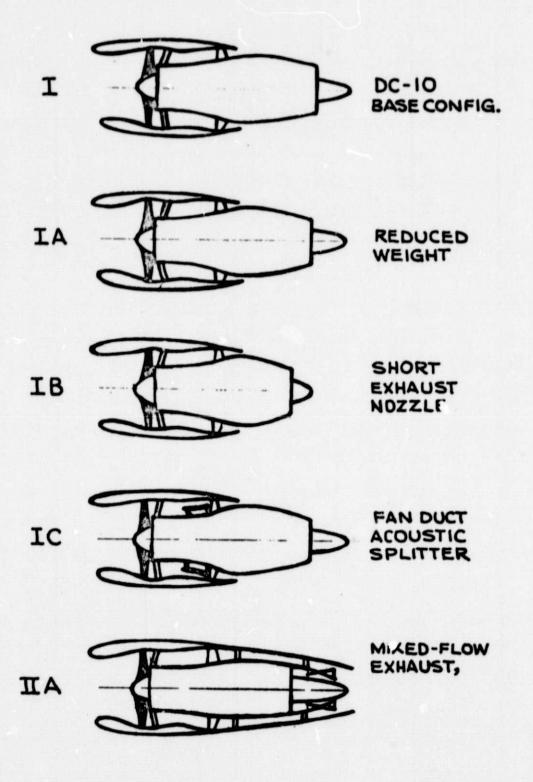
FIGURE 4. - DOUGLAS STUDY CONFIGURATIONS FOR WIDE BODY TRANSPORT
