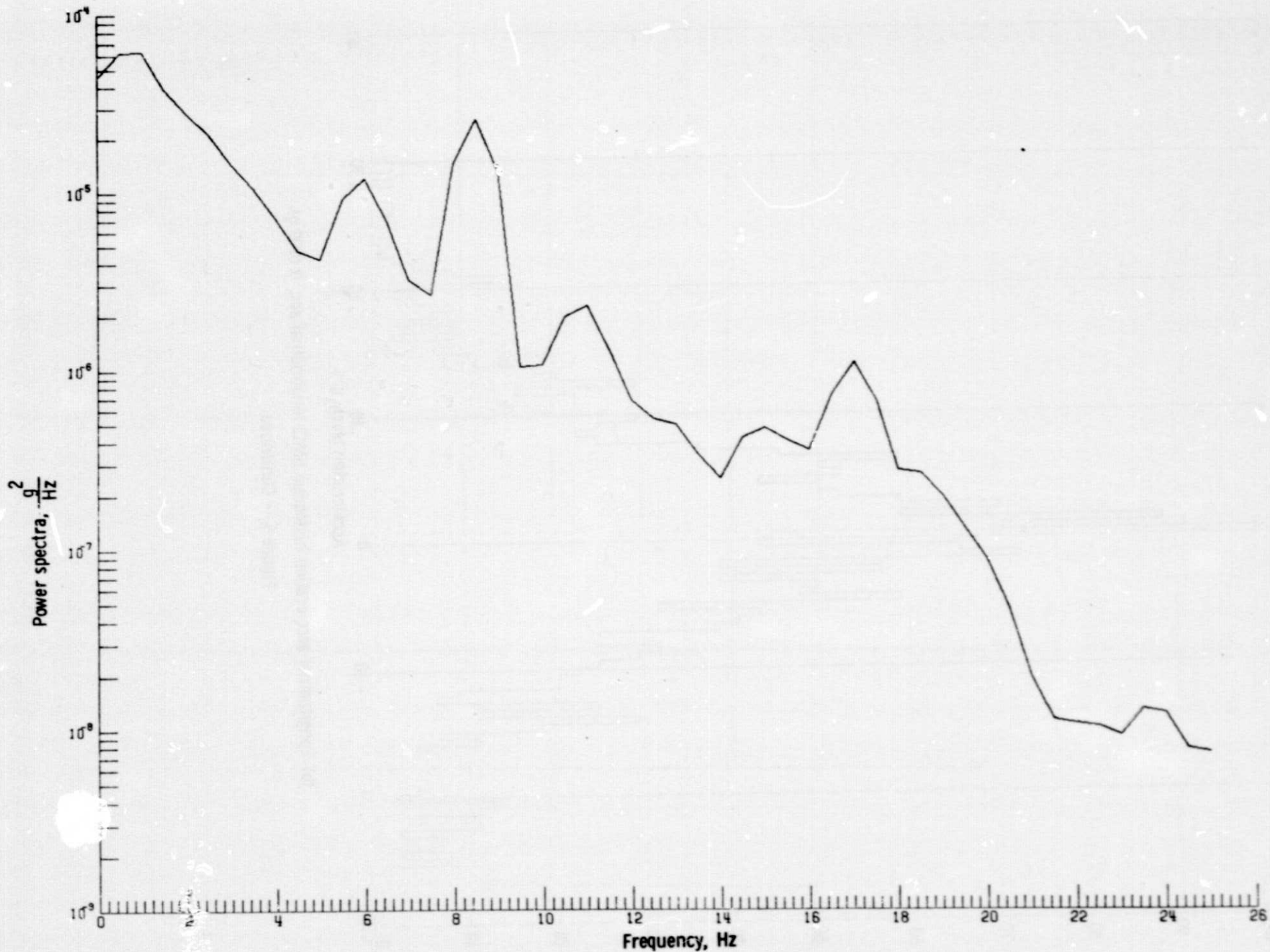
(c) Longitudinal acceleration power spectrum (RMS longitudinal acc. 0.0141 g).
