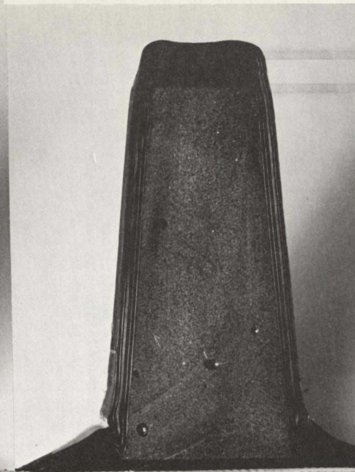
FIGURE 28b. CROSS SECTION VIEW OF FRAME LAMINATE EWR-39411-042 SPECIMEN #2 SHOWING WEB LAMINATE BULGES AT BASE OF FOAM.
