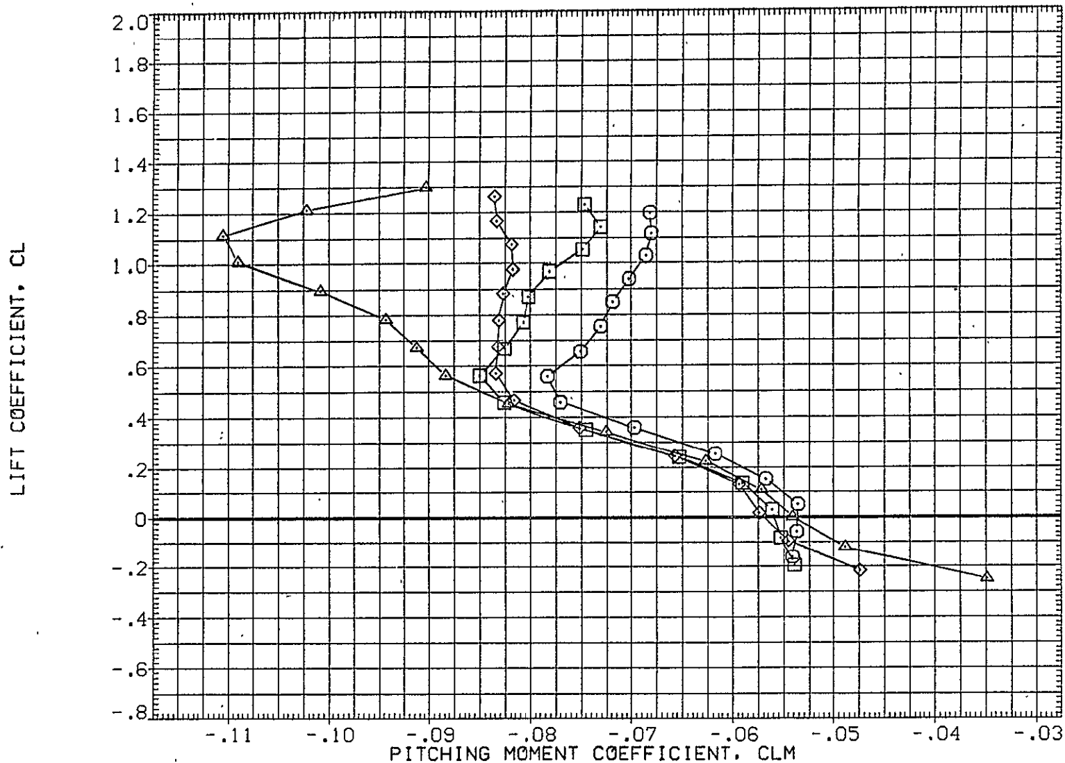
FIG. 32 747+ORB(10 DEG)+SP45,HORIZ OFF, FLAPS 20 LAUNCH
