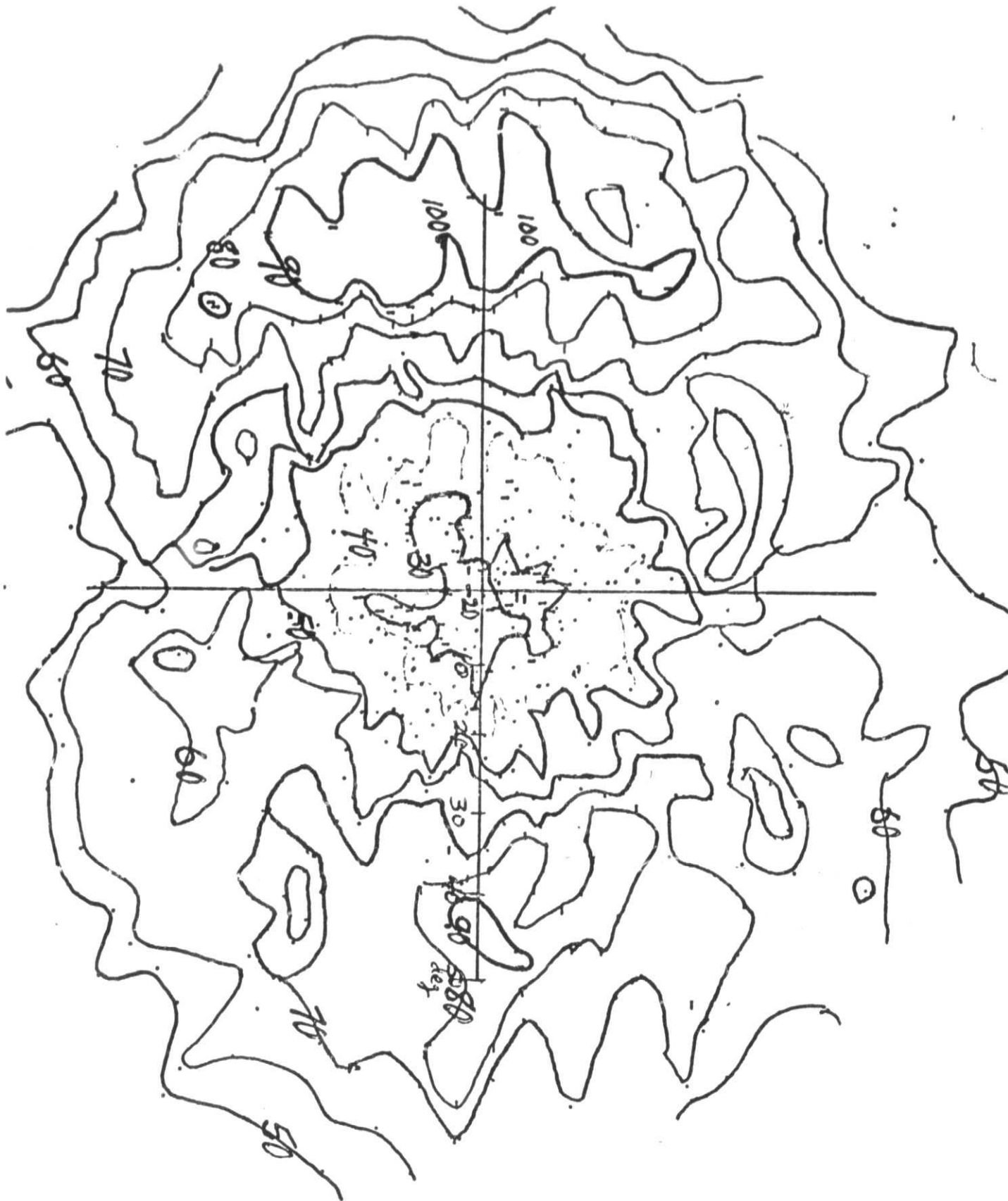
Figure 18 - (10.0) pole figure for annealed commercial titanium sheet.
