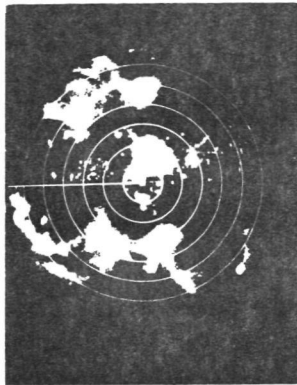
Fig. 2. 10 GHz PPI display showing at least seven clearly discernible rain cells in Columbus, Ohio, USA. The range rings are at 2 mile intervals. The small discrete echoes are ground clutter.
