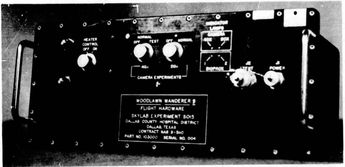
Figure 1.- External configuration of S015 flight unit.
