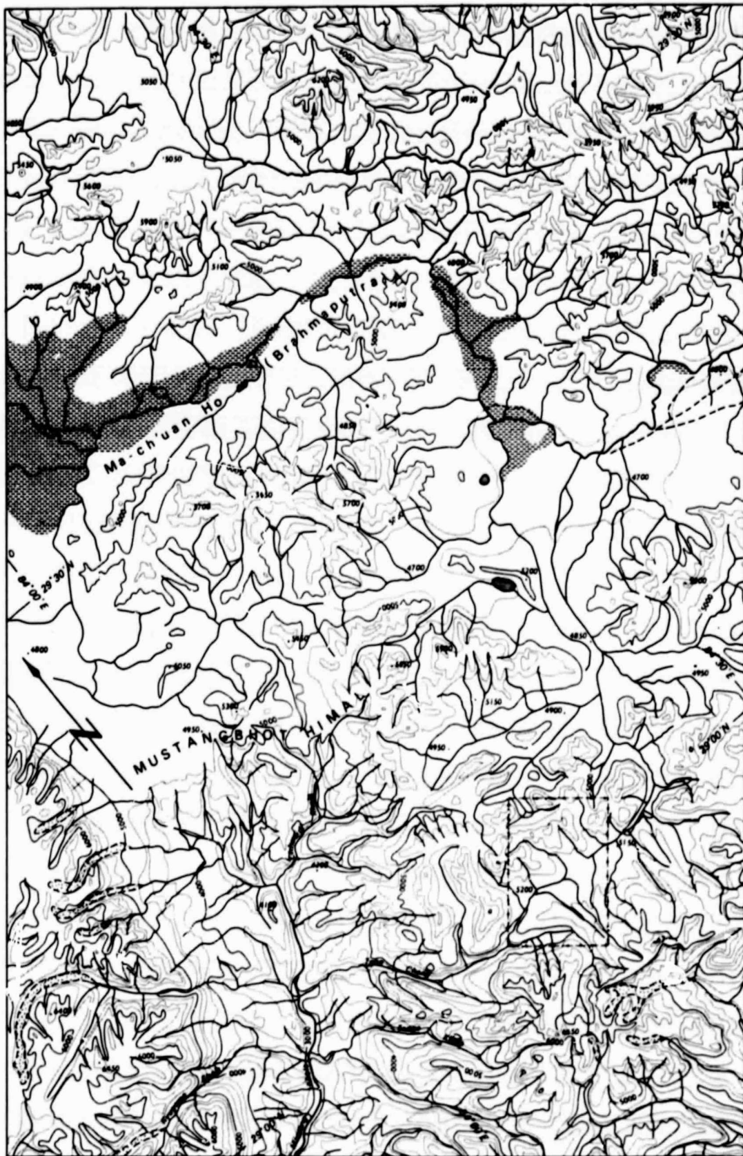
Figure 7. Photogrammetric map plotted from multispectral camera photography at a scale of 1:500,000 with contours at 250m. V.I.
