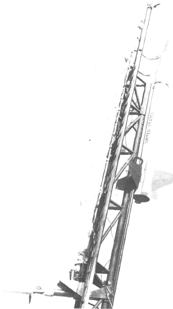
Figure 4.- Test vehicle mounted on rail launcher.
