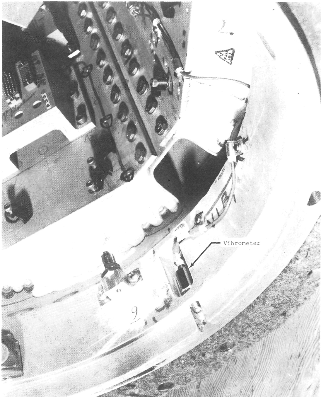
Figure 7.- Vibrometer on forward motor ring (view looking forward).
