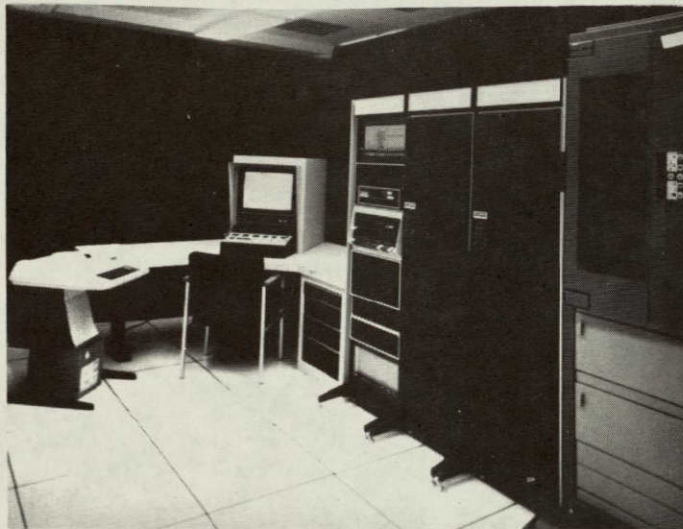
Figure 2. Computer Generation of Land-Use Maps from LANDSAT Data. The Datagrid is Used to Digitize Ground Control Points and Boundaries of Areas for Which Area Tables are Required. M-DAS Transforms the Datagrid and LANDSAT Computer Tapes into Area Tables, Categorized Map Overlays, Color-Categorized Imagery, and Rescanned-Resampled Tapes.
