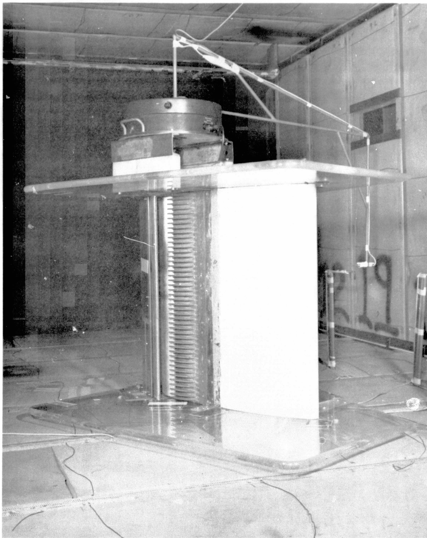
FIGURE 1. MODEL SCALE AUGMENTOR WING IN TUNNEL TEST SECTION
