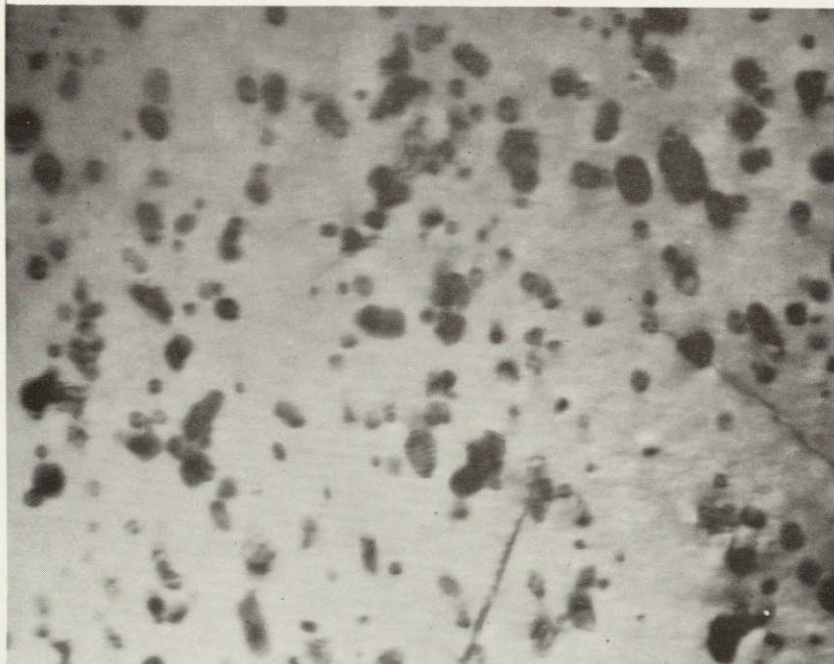
Figure 27: Dispersoid observed in extrusion 201HC - nominal composition \text{Ni-16Cr-6Al-1.2Y}_2\text{O}_3 - magnification 20,000X
