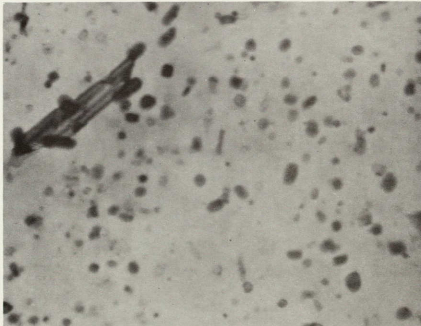
Figure 23: Dispersoid observed in extrusion 197LA - nominal composition Ni-16Cr-4Al-1.2Y 2 O 3 - magnification 20,000X
