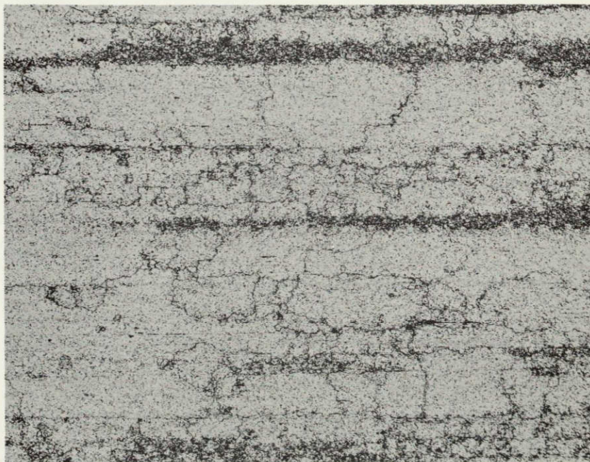
Figure 13: 199HB - furnace recrystallized - in at 1478°K (2200°F) → 1616°K (2450°F)/1 hour - magnification 100X
