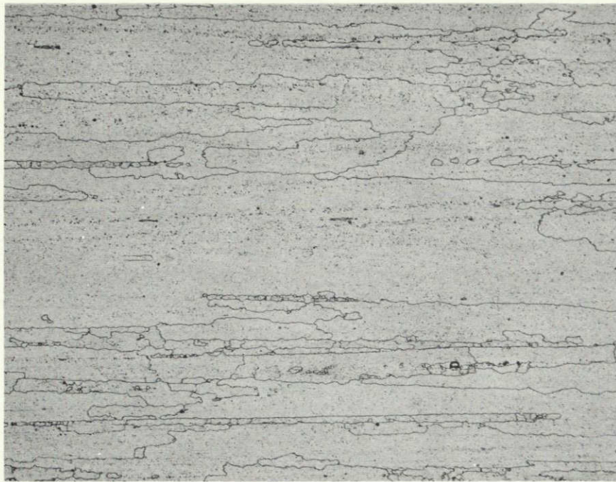
Figure 18: 198LB - furnace recrystallized - in at 1616°K (2450°F)/ 1 hour - magnification 100X
