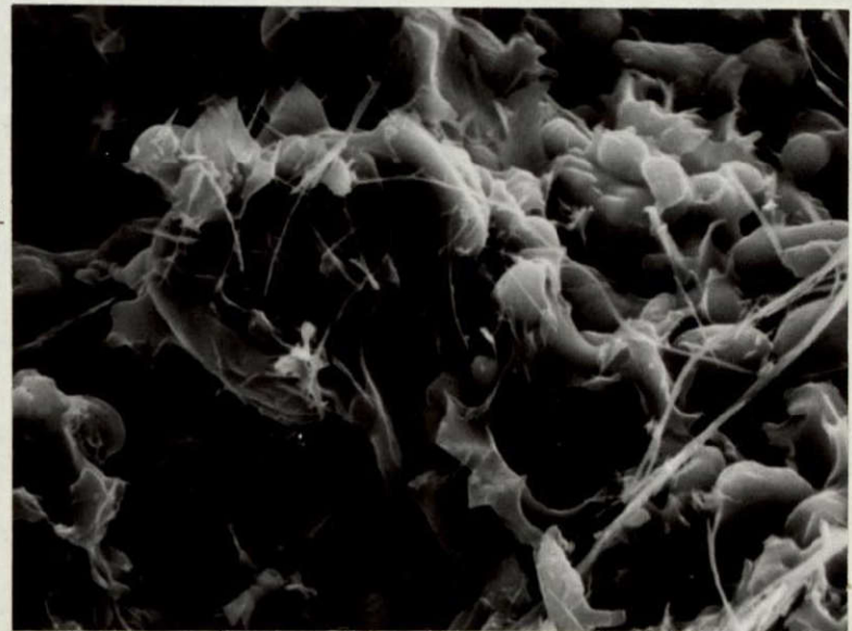
FIGURE 21. Two magnifications of Sample #554D3 and #554D4, both with 70% Al, tested at 25° and 250°C, respectively. Shear strength dropped from 3715 psi to 2335 psi. Higher filler content increases the fracture-surface area and prevents the 'melting' at high temperature. Fibers are artifacts.
