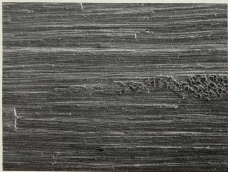
FIGURE 18. Two magnifications of opposite mating fracture surfaces from Sample #948D1; one adherend was titanium and the other was HT-S /P13N composite molded at 400 psi. Shear strength was 3750 psi and failure was mostly in the composite.
