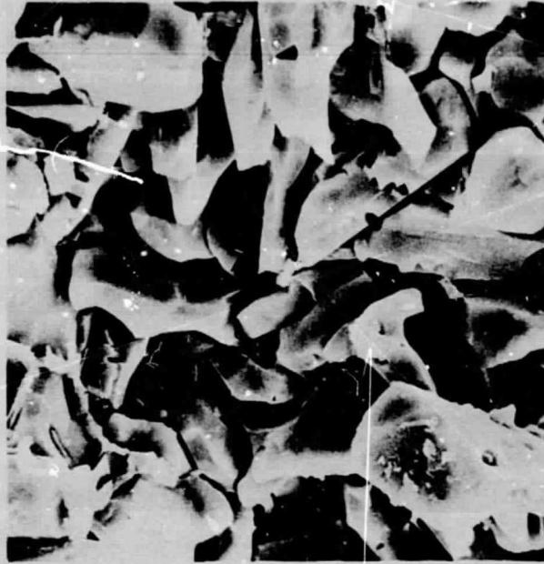
Figure 14. SEM Photomicrograph of Ceralloy 146A SiC - Treated in a \text{CaCl}_2 - \text{CaF}_2 - \text{CaSO}_4 molten salt bath at 830^\circ\text{C} for 30 minutes. 2000X
