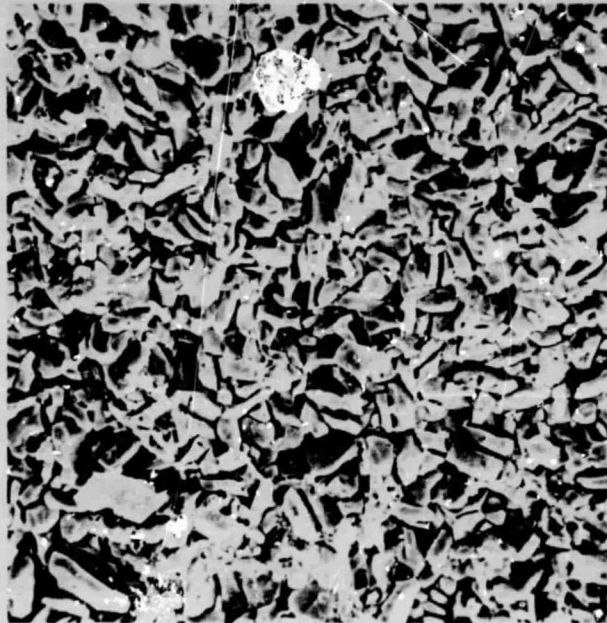
Figure 13. SEM Photomicrograph of Ceralloy 146A SiC - Treated in a \text{CaCl}_2 - \text{CaF}_2 - \text{CaSO}_4 molten salt bath at 830° C for 30 minutes. 500X
