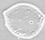
Figure 8. Specimen No. IHP3 Thermal- etched at 1500°C - (1 mm = 3.8 μm) 263X
