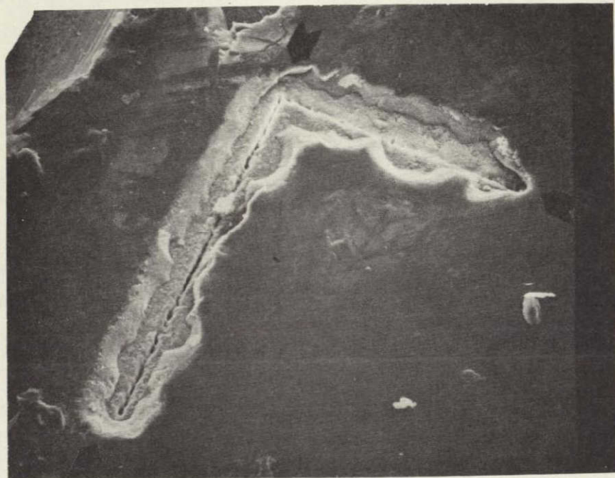
Figure 2. Laser-trimmed thin film resistor through DC 62-047 WE silicone coating (SEM photo at 162X).
