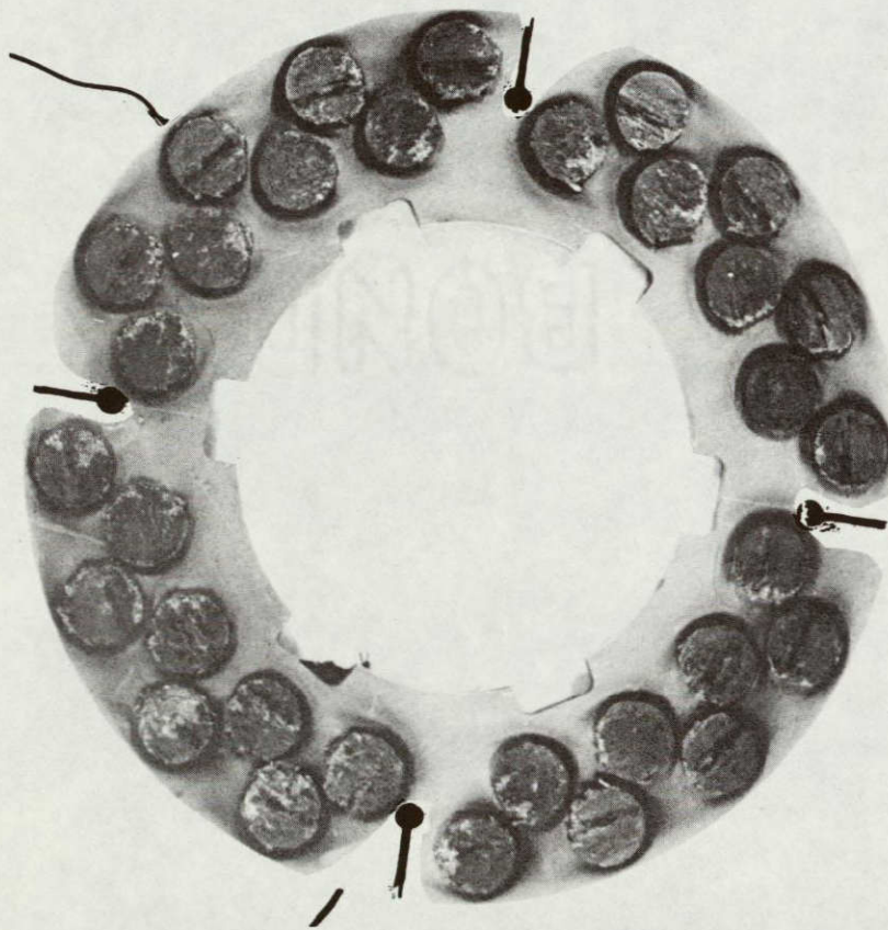
Figure 15 Photographs Showing the Rubbed Surface Conditions of Stators, One with Mo/LPA Buttons and the Other with Nickel-Based Buttons after all Evaluation Tests
