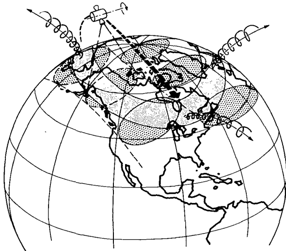
FIGURE 1.—Schematic illustration of the geometry for observing the bremsstrahlung associated with electron precipitation at high latitudes. The shaded ellipses indicate schematically the fields of view of the spectrometers for different positions of the spinning satellite, and the shaded "band" indicates schematically a region from which bremsstrahlung is observed.
