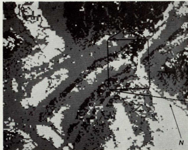
A. Gray scale coded PHOTO image. (White = alluvium, gray = shale, black = sandstone.) Approximate scale of original 1:150,000.
