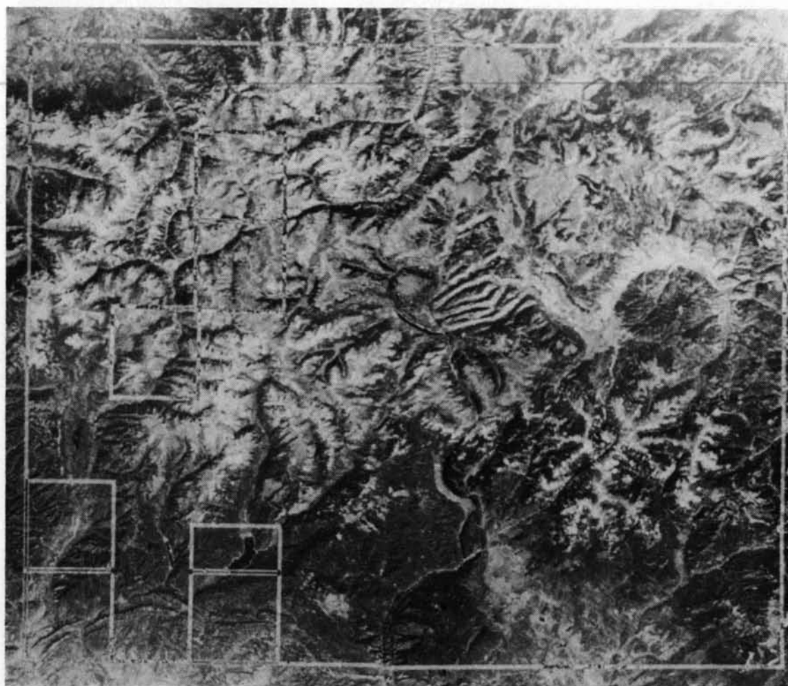
Figure A.19. ERTS-1 MSS Band 5 (0.60-0.70um) grayscale image (frame 1425-17190) of the San Juan Mountain test site showing the location of the quadrangles used in the areal comparison evaluation.
