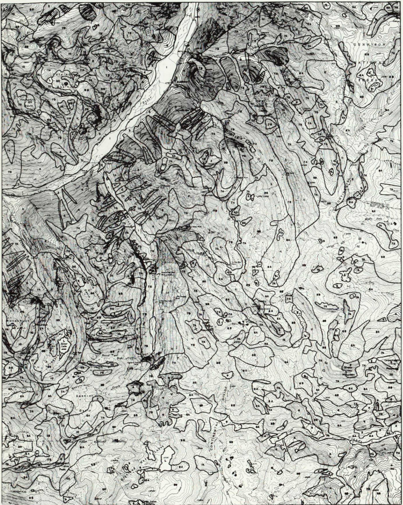
Appendix C.5 Figure. Geomorphic characteristics for Howardsville quad derived through interpretation of NASA underflight photography.
