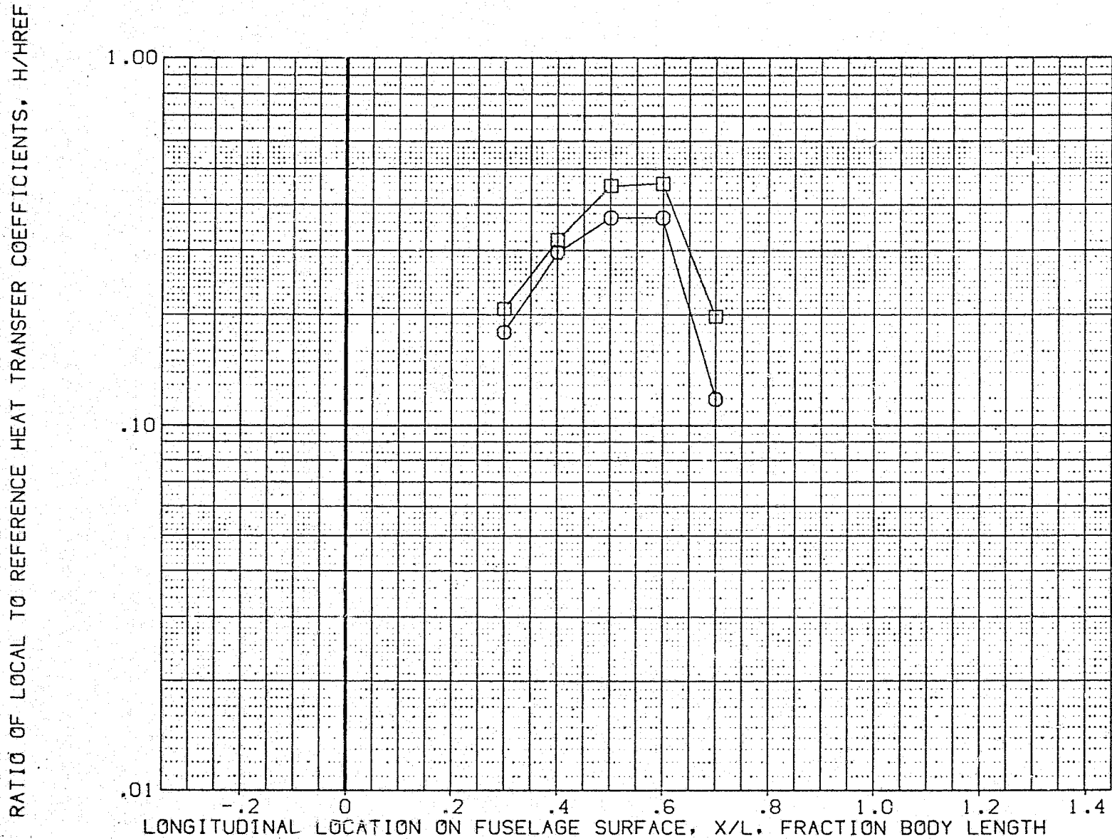
FIG 10 FUSELAGE SIDEWALL AND UPPER SURFACE DISTRIBUTION VAR.W/SIDESLIP ANGLE
