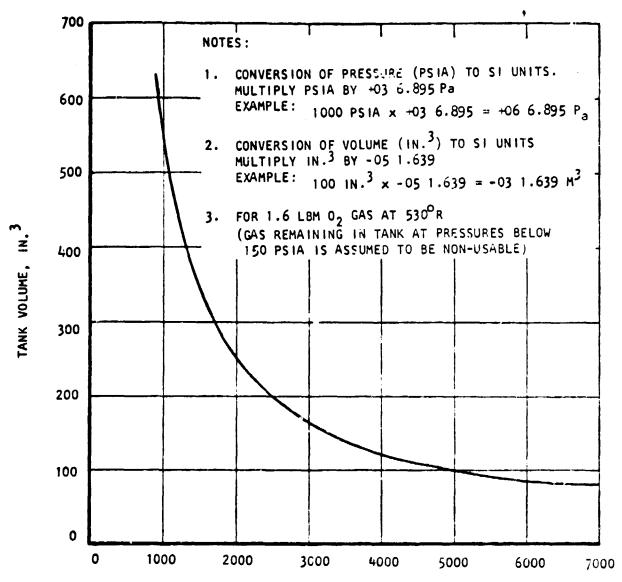
Figure 3-1. Tank Volume vs. Tank Pressure Needed to Provide 1.6 Lbm Usable  $\mathbf{0}_2$  Gas
