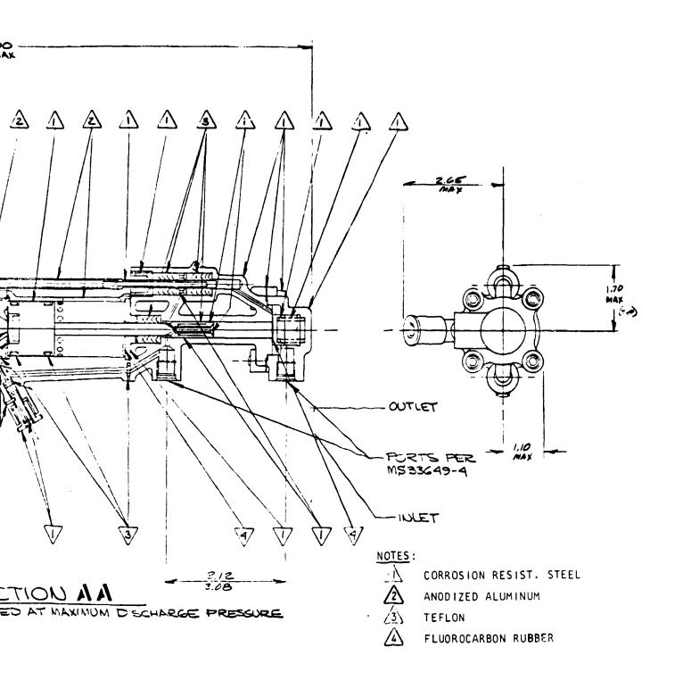
Figure 4-2. Initial Prototype Pump Design
