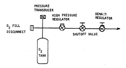
In this schematic, the high pressure regulator and all hardware upstream would be subjected to tank pressure. This includes the oxygen fill disconnect, pressure transducer, tubing, and regulator. Each item is evaluated in the following paragraphs.
