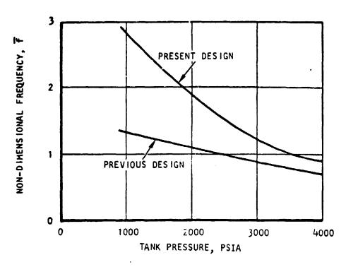
Figure 4-6. Non-Dimensional Frequency for Previous and Present Designs
