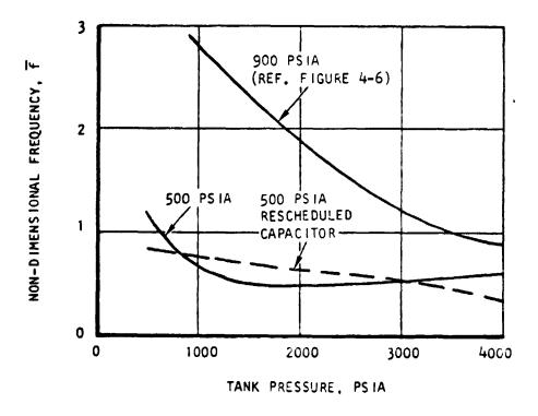
Figure 4-7. Non-Dimensional Frequency for 500 psia Supply Pressure
