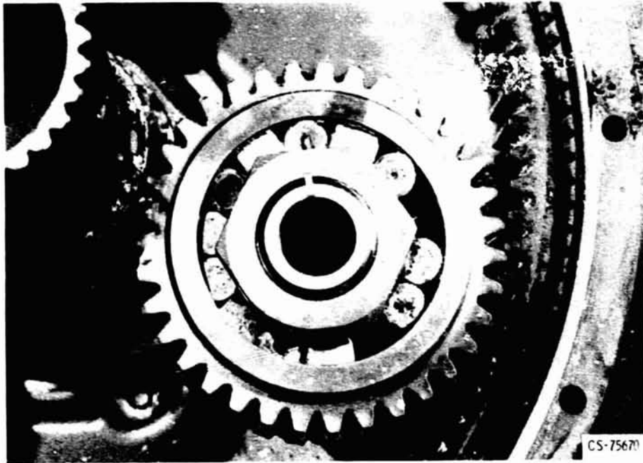
Figure 11. - Planet gear support bearing. Badly misaligned and skewed rollers caused high vibration and temperature levels.
