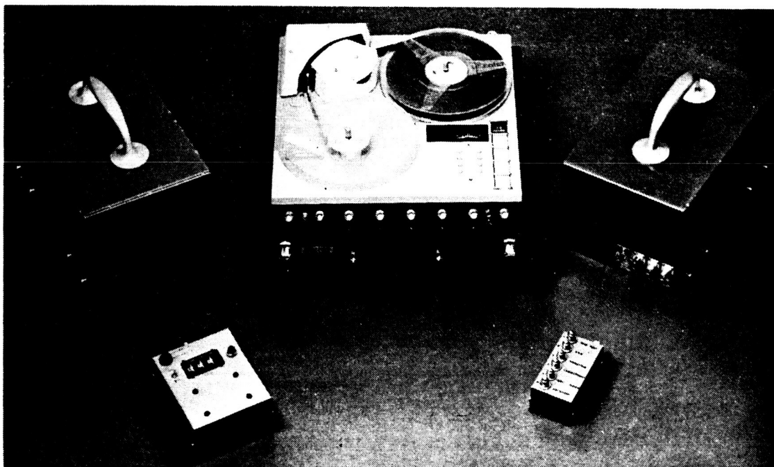
Figure 1.- Vibration measuring and recording system.
