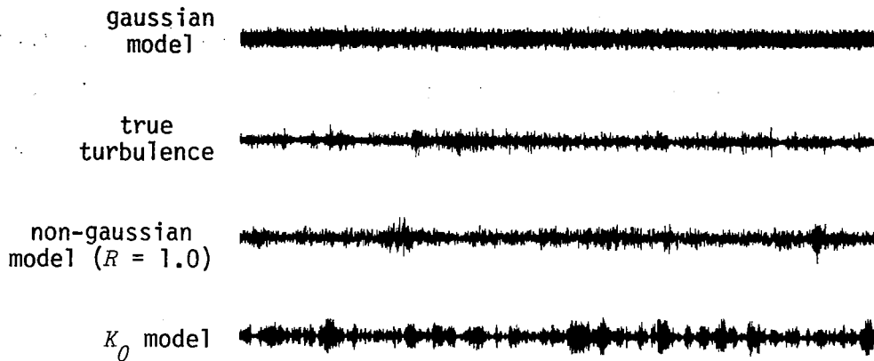
Figure 10.--The derivative of an atmospheric turbulence sample compared with derivative samples from several turbulence models. Sample length for these data is approximately 11 kilometers.
