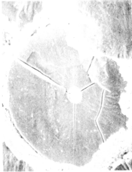
FIG. 41 -- SEM photographs of fracture of specimen DP 28B after 1800°F tensile test. Note matrix/filament interaction (arrows) (fiber lot 8S80 HIP at 1825°F)
