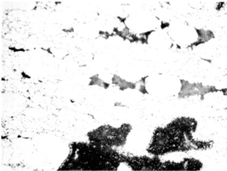
FIG. 26 -- Waspaloy HIP consolidated at 1038°C (1900°F). Tensile tested at 982°C (1800°F). Longitudinal section near fracture
